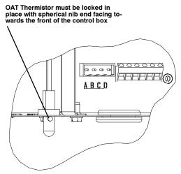
Fig. 8 - Outdoor Air Thermistor (OAT) Attachment
